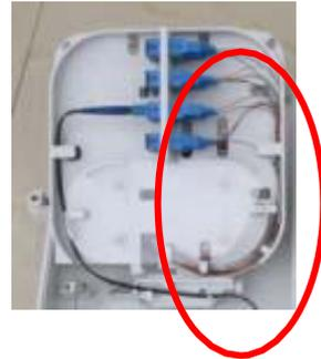
7. Insert optical drop cables to the outlet holes, then seal the holes to provide a water tight seal.
